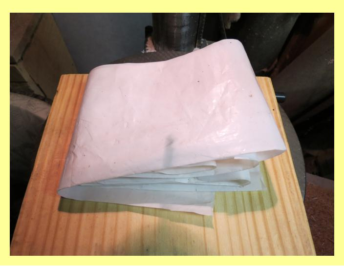
Use hot glue to fasten the plastic inside the lid. This is a barrier to keep the spray dripping inside the tote.
